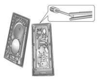
2. Use the key blade to separate the two halves of the transmitter.
